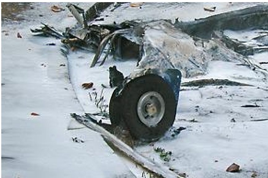
Fig. 6: Scorched tyre of the right wheel
